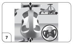
Align the steering wheel with smaller front wheels, so that wide end of the steering wheels faces forward. When front wheels are unassembled and resting on a flat surface, the smaller front wheels do not contact the ground.
