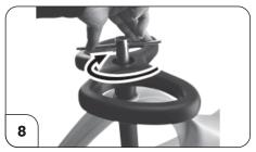
This step is critical to the performance of your swing car. Use a 17mm socket wrench to tighten the nut in the steering column as tight as possible. You can also use the included hex key tool.
