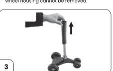
Remove the foam sheath from the front wheel assembly.
