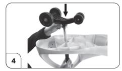
Guide the front wheel shaft through the body, into the foam sheath, and through the hole at top of body.
