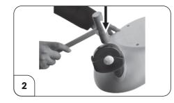
Strike the rear wheels with a rubber mallet to secure them into place.
