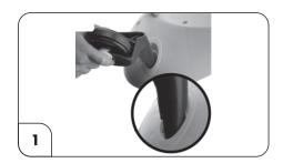
Fill the notch on each rear wheel housing into the body. Push the wheels in 45 degree angle. When installed correctly, the rear wheels flare out from the body. Once locked into place, the rear wheel housing cannot be removed.
