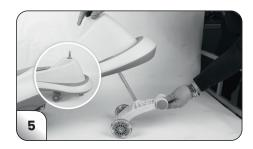
Insert the front wheel to the end, and the front wheel bearing is fully locked into the car body.
