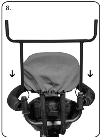
8. Insert T-frame into the backrest.
