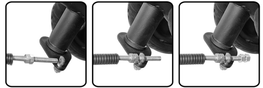
10. Inset the hook shaped rod in the front (just above the mudguard) and tighten it using the nut in the back side, as shown in the picture. The alignment of front handle & parental control can be done by adjusting the nuts on the movement bar.
