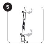
Pull back both the clamps on the handle and footrest to unlock the handle of the scooter.
