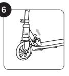
Pull the lever on the footrest and bend the handle of the scooter to fold and store easily
