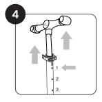
Push the button and press the handle up or down to adjust it as per the desired height.
