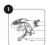
Pull the lever to loosen the clamp and lift it to unfold and open the scooter.
