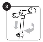
Insert the handle into the scooter till you hear a click. Pull back both the clamps on the handle to lock it in place.
