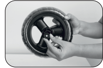
11. After inserting a small rod from front side, put the second vicer into the same as shown in picture
