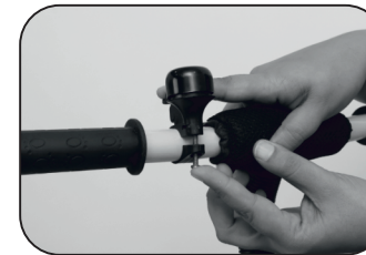
16. Install the bell with the help of screw
