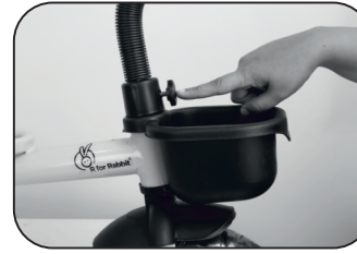
6. Tighten up the fork screw given as shown in picture
