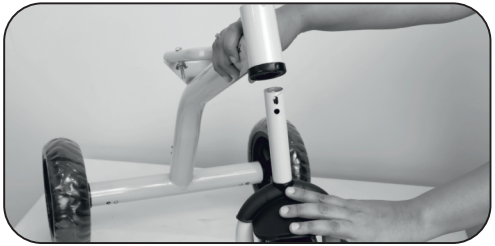
3. Insert the main body into front ones post fitting with round black vicer given.
