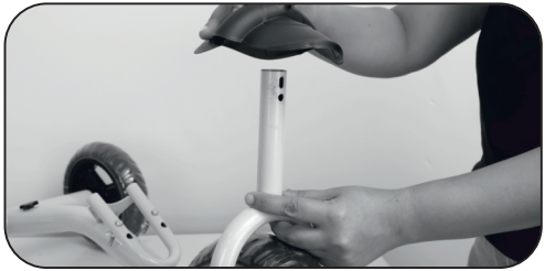
2. Install the mudguard into the front body of tricycle as shown in ref pic
