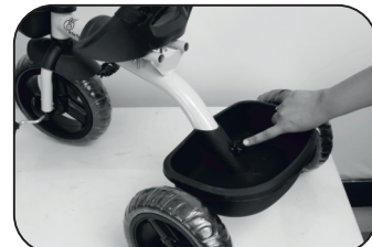
15. Fix the rear basket and tighten the same with the help of fork screw
