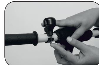
16. Install the bell with the help of screw
