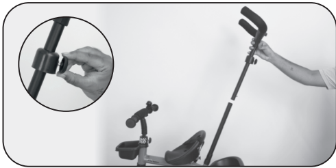
19. Install the parental control and tighten the same with fork screw
