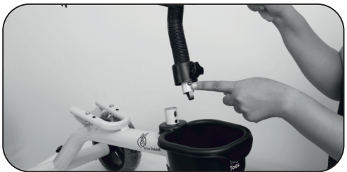
5. Install the front steering part with the help of push pin given on both the sides (Front and Back Side)
